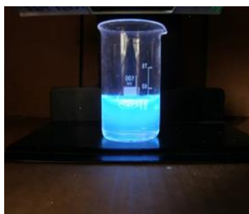
Figure (6). An image of a carbon quantum dot particle sample under UV-light.
