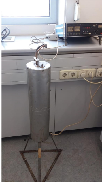
Figure 5: Heating sample at 500 o C in Electric Furnace for 30minutes
