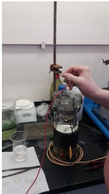
Figure 7: Electro polishing the sample
