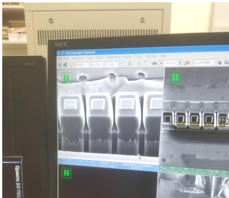
Figure 10: Ones of the fabricated micro pillars (each pillar is 15 \mu m long and square side of 5.25 \mu m)
