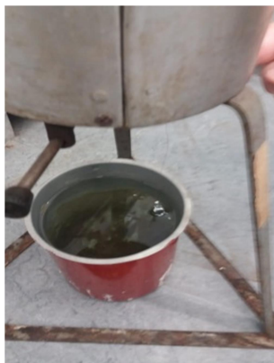
Figure 6: Quenching the Sample in water at Room temperature
